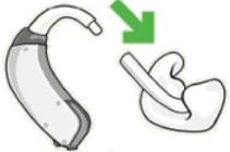
Disconnect the hearing aid by pulling it apart at the connection between the hook and tubing
