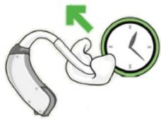
Wait until the earmould is completely dry before connecting it back together
