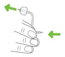
Push the tool all the way through until it comes out of the dome end
