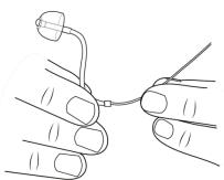
Insert the cleaning tool in the tube
