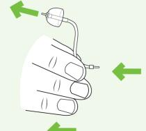
Push the tool all the way through until it comes out of the dome end.
