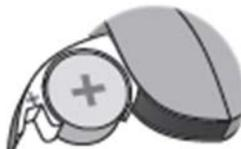
Insert the new battery into the battery drawer with the + side facing upwards.
