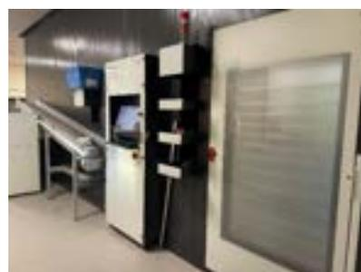
The previous system was 16 years old, and is replaced by a more modern, more efficient robot. Once Pharmacy staff process the label for the medicine or input an order for stock, the robot selects the box from the shelves, scans it to ensure it is the right medication and transports it along a conveyer belt to a collection point.
