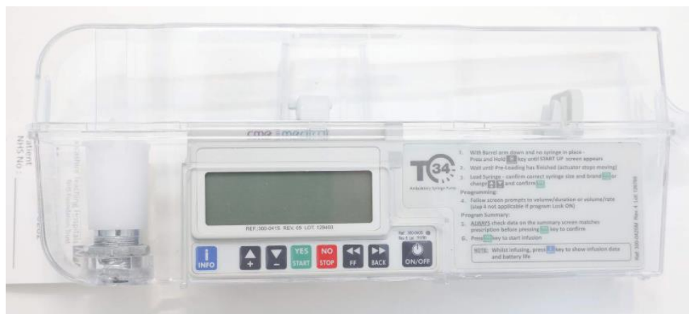
A syringe driver infusion pump
